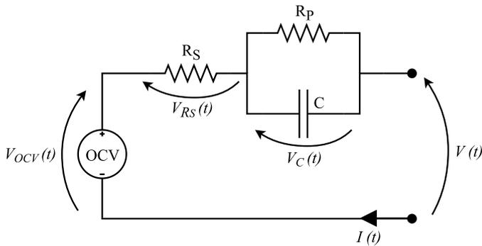
Fig. 1. Thevenin equivalent model of the battery.
