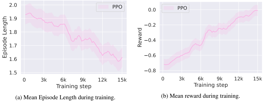
Figure 12: RoboFeeder-picking-v0, PPO training curve of mean episode length and reward over 5 seeds.
